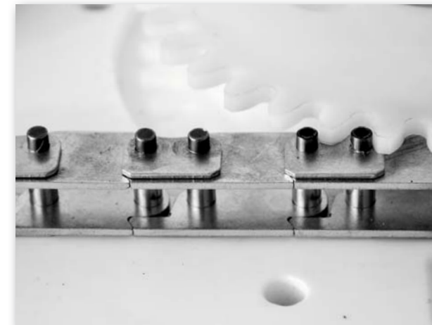
Catene tiro e spinta (attuatore) Push and pull chain (actuator)
