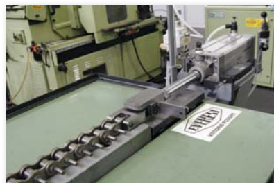
Banco misurazione Chain measuring bench
